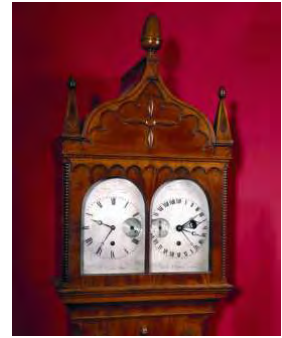
Solar and sidereal time clock. Sidereal dial shows 24 hours with the two lower hands, and a third, large hand shows phases of the moon and its position relative to the sun, which is represented by the fourth hand above. Science Museum, London
